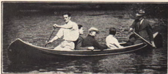
16-foot "Sponson" Canoe carrying five persons (800 lbs.). No overload. Note the good freeboard.
