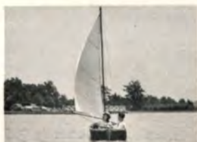
Linkboat equipped with sectional sailing rig complete with standard type keel, rudder, etc.
