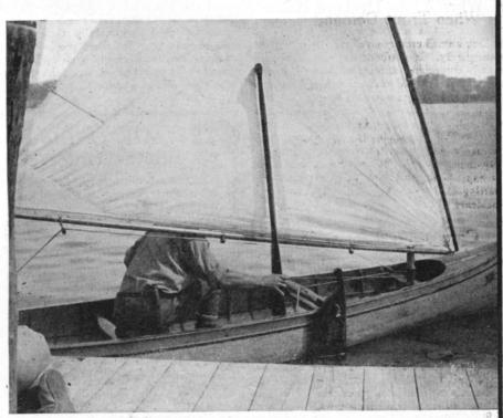
This shows, roughly, the center of effort. The top of the paddle must be over, or, correctly, six inches aft the center of lateral resistance, with the weight in the center of the canoe, to assure its full sailing possibilities.
